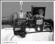
TYPICAL 1. Engine start button 2. Engine stop switch **NOTE:** The engine will not turn if the engine stop switch is turned to OFF position.
